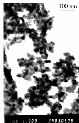
Fig.5 TEM image of nanoscale \text{In}_2\text{O}_3 powder
