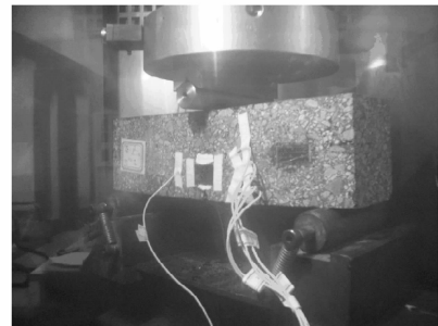
Fig. 6 Crack propagation gauge bonded on the specimen
