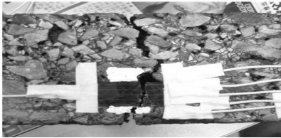
Fig. 9 Debonding mechanism of AK-13B fatigue fracture
