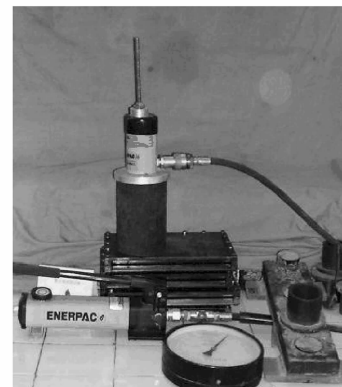
Fig. 5 Pulling-out test machine and samples
