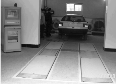
Fig. 1 4PLD test rig for vehicle braking vs. suspension anti-vibration efficiency
