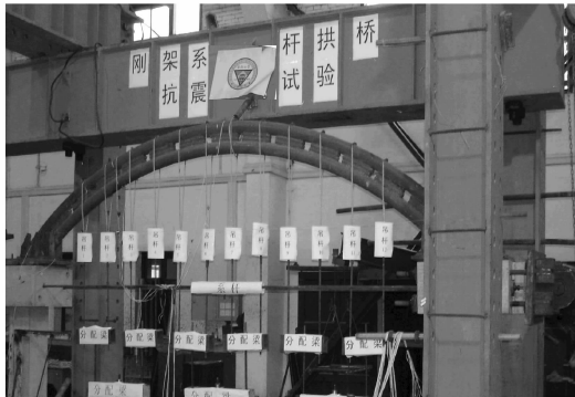
Fig. 2 Test setup and details of test specimens. (a) Schematic test setup (cm); (b) Elevation (cm); (c) Cross section 1-1 of common piers (mm); (d) Cross section 1-1 of split-piers (mm); (e) Cross section 2-2 (mm); (f) Picture of test setup
