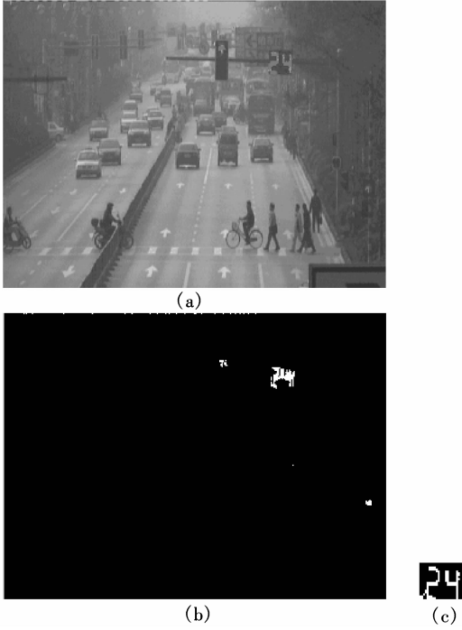
Fig. 2 Detection of red traffic lights. (a) Intersection traffic light; (b) Traffic light detection; (c) Character extraction
