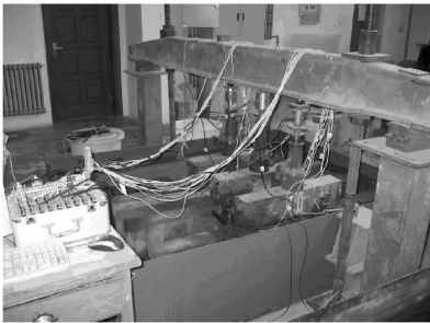
Fig. 3 Beams under sustained load and wet-dry saline water
