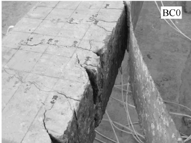
Fig. 6 Failure of controlled beam(BC0)
