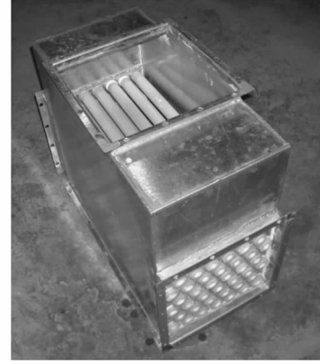
Fig. 1 Photo of the porous ceramics tube type dew point indirect evaporative cooler
