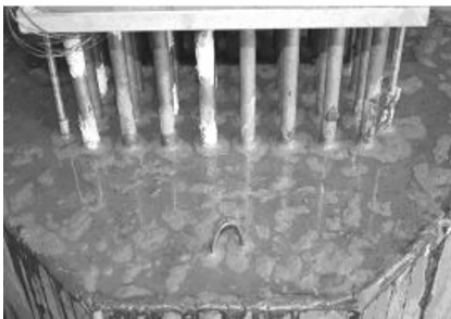
Fig. 2 Centrifuge test model of pile groups
