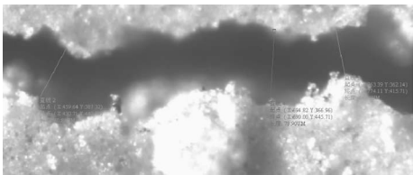
Fig. 3 Crack width measured by optical microscope (Crack widths are 60, 78 and 54 \mu\text{m} , respectively)
