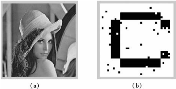
Fig. 5 Simulation results of the contourlet + Arnold + SVD algorithm. (a) Image with watermark; (b) Extracted watermark image
