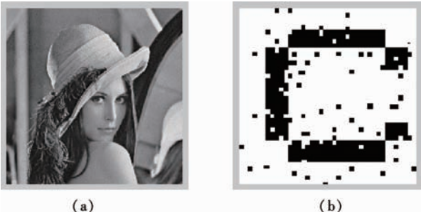
Fig. 4 Simulation results of the contourlet + SVD algorithm. (a) Image with watermark; (b) Extracted watermark image
