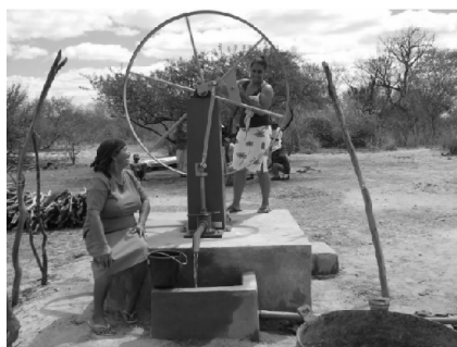
Fig. 6 Volanta hand pump with a fly wheel takes water out from cracks in the crystalline subsoil (Irpaa)
