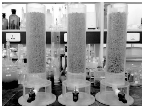
Fig. 1 Permeation columns used for dynamic adsorption experiment
