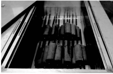
Fig. 2 Specimens immersed in the temperature-controlled tank
