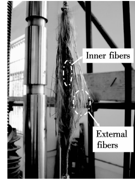
Fig. 6 Typical failure mode of BFRP bar of group A (120 d exposure)
