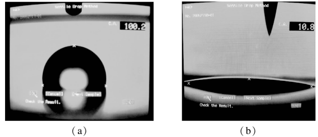
Fig. 6 Contact angles of different interfaces. (a) YC-1005G-NT and water; (b) YC-1005G-NT and asphalt
