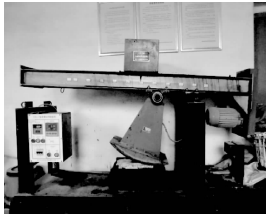
Fig. 5 Ice on surface of specimen compressed by rut board molding pendulum
