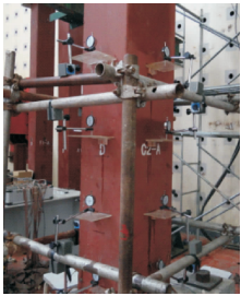
Fig. 4 Location of displacement meters
