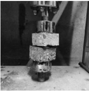
Fig. 4 Pull-out test equipment
