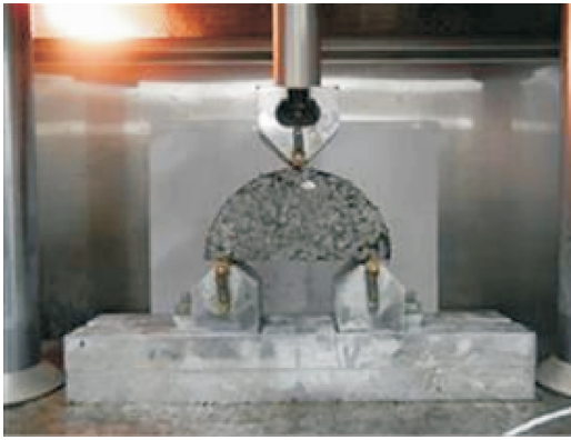
Fig. 1 SCB test setup
