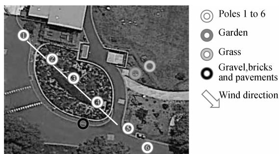
Fig. 3 Plan view of Fitzroy Raingarden microclimate observation gear
