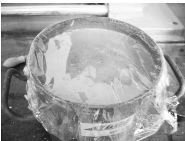
Fig. 3 Bleeding measurement
