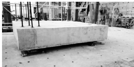
Fig. 6 Concrete slab block for shaking table tests
