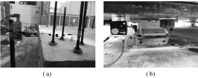
Fig. 9 Layout of measuring instruments. (a) Wire-type displacement transducer; (b) Three-direction accelerometer
