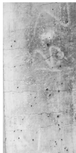
Fig. 4 Multiple cracks of bending HS-HDCCs specimens with PE fibers
