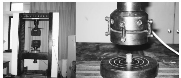
Fig. 1 Unconfined uniaxial compression physical test
