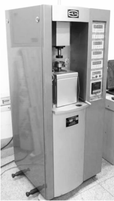
Fig. 5 The pin-on-disc tribometer
