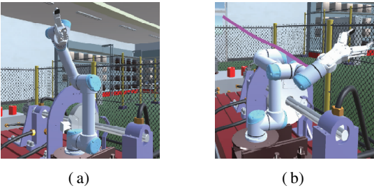
Fig. 20 Simulation results of the robot arm trajectory planning in the virtual environment. (a) Initial posture; (b) Termination posture
