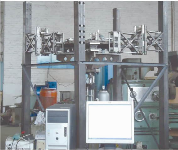
Fig. 9 Experimental shake table with VSMs
