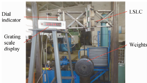
Fig. 5 Equivalent stiffness measurement of the LSLC
