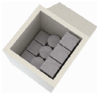
Fig. 4 Arrangement of the concrete specimens inside the incubator
