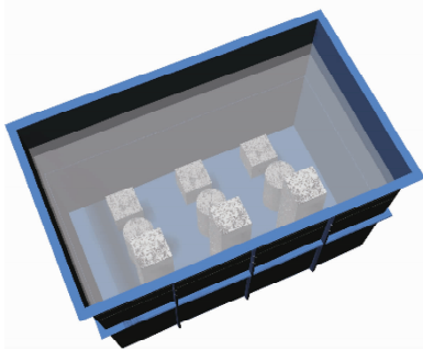
Fig. 3 Arrangement of the concrete specimens inside the water tank
