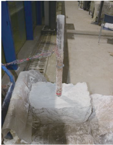
Fig. 1 Rock-socketed pile model made of phosphogypsum for simulating the rock
