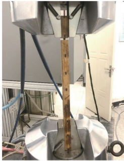
Fig. 3 Test setup for the pull-out test
