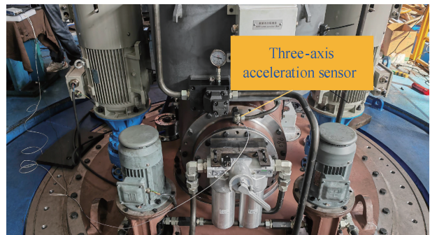
Fig. 7 Marine rudder propeller slewing bearing test bench
