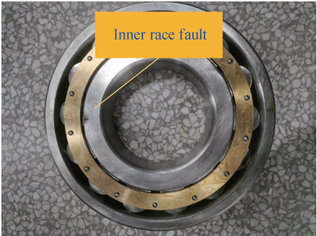
Fig. 8 Inner race fault
